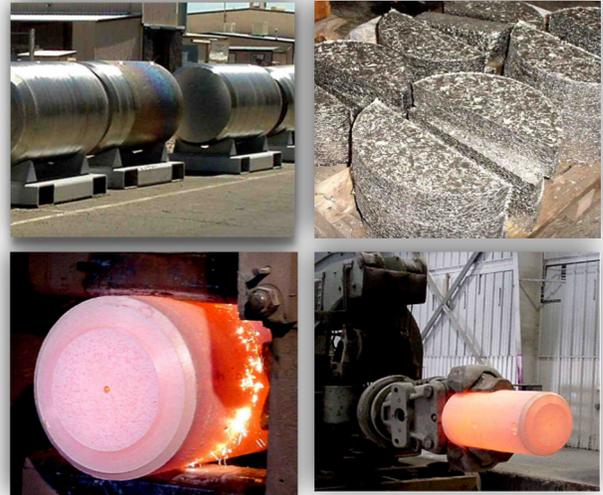
*The zirconium ingots in the top left image can be shipped, as is, to customers. Others await further processing at WZ through many production techniques available— forging, extrusion, melting, rolling, chemical baths, annealing, lathing/cutting.*
